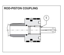
The rod and piston are mechanically cou-Ine rod and piston are mechanically coupled by a threaded connection in which the thread on the rod is at least equal to the external thread KK, indicated in the table [7]. The piston is screwed to the rod by a prefixed tightening torque in order to improve the fatigue resistance. The stop pin ① avoids the piston unscrewing the piston unscrewing.
