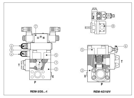
REM are double stage pressure relief valves with balanced poppet and SAE flange connection, designed to operate in oil hydraulic systems.
