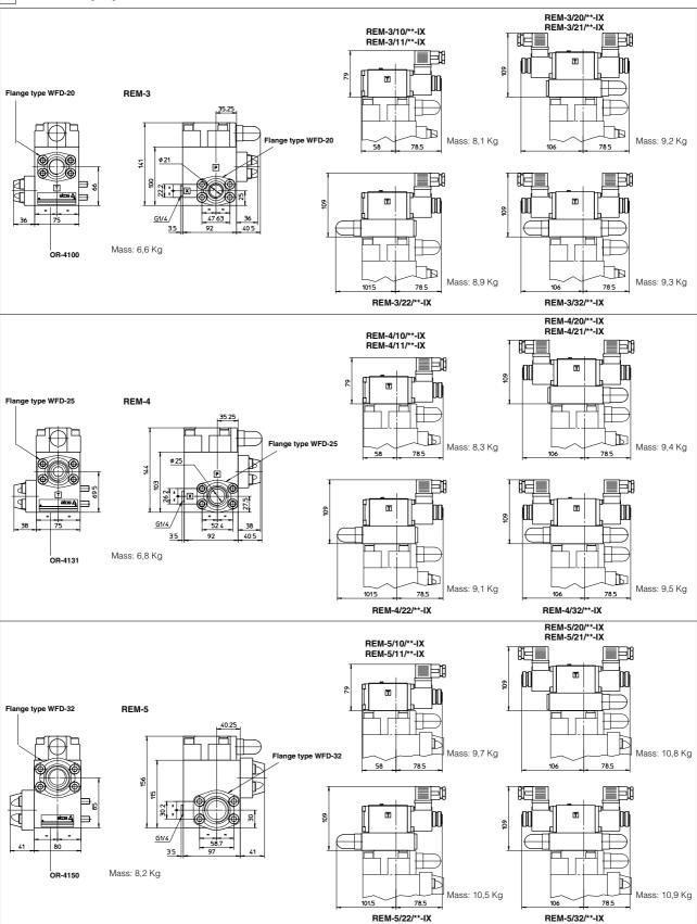
For dimensions of flanges, see tab. K120. Overall dimensions refer to valves with connectors type SP-666.
