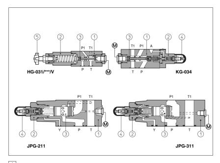
HG, KG, JPG are pressure reducing valves, spool type 3, designed to operate in oil hydraulic systems.
