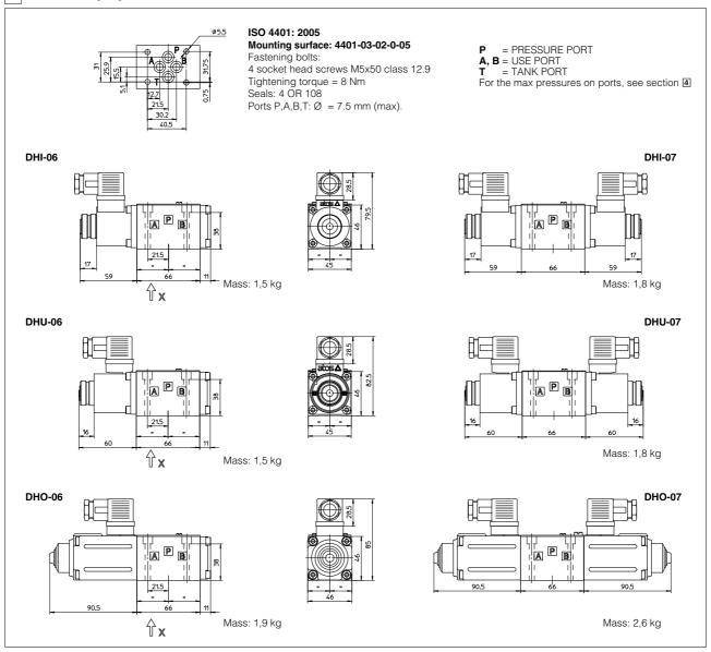
Overall dimensions refer to valves with connectors type SP-666
