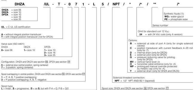
**L** = linear; **S** = progressive; **D** = as **S**, but with P-A = Q, P-B = Q/2(1) Option **/BT** = low temperature -40°C also available on request
