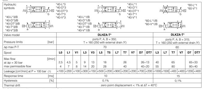
(1) Referred to spool in center position and 50°C oil temperature.
