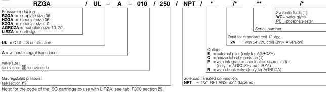
Note: for the code of the ISO cartridge to use with LIRZA, see tab. F300 section [2]. (1) Option **/BT** = low temperature  $-40^{\circ}$ C also available on request
