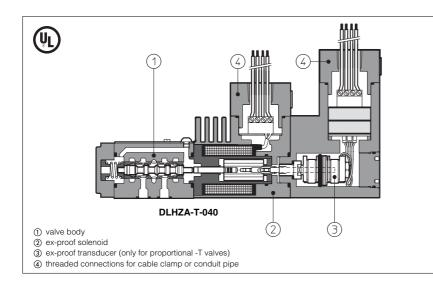
Explosion-proof on/off and proportional solenoids certified C UL US according to UL 1002 and CSA 22.2 n°139-1982 Standard, Class I, Groups C&D (Groups IIA & IIB to NEC 505-7).
