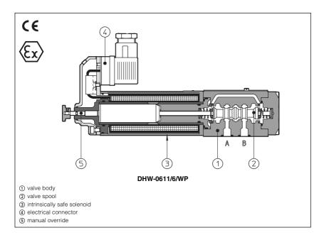
On/off valves equipped with intrinsecally safe solenoids certified according to ATEX 94/9/CE, protection mode:
