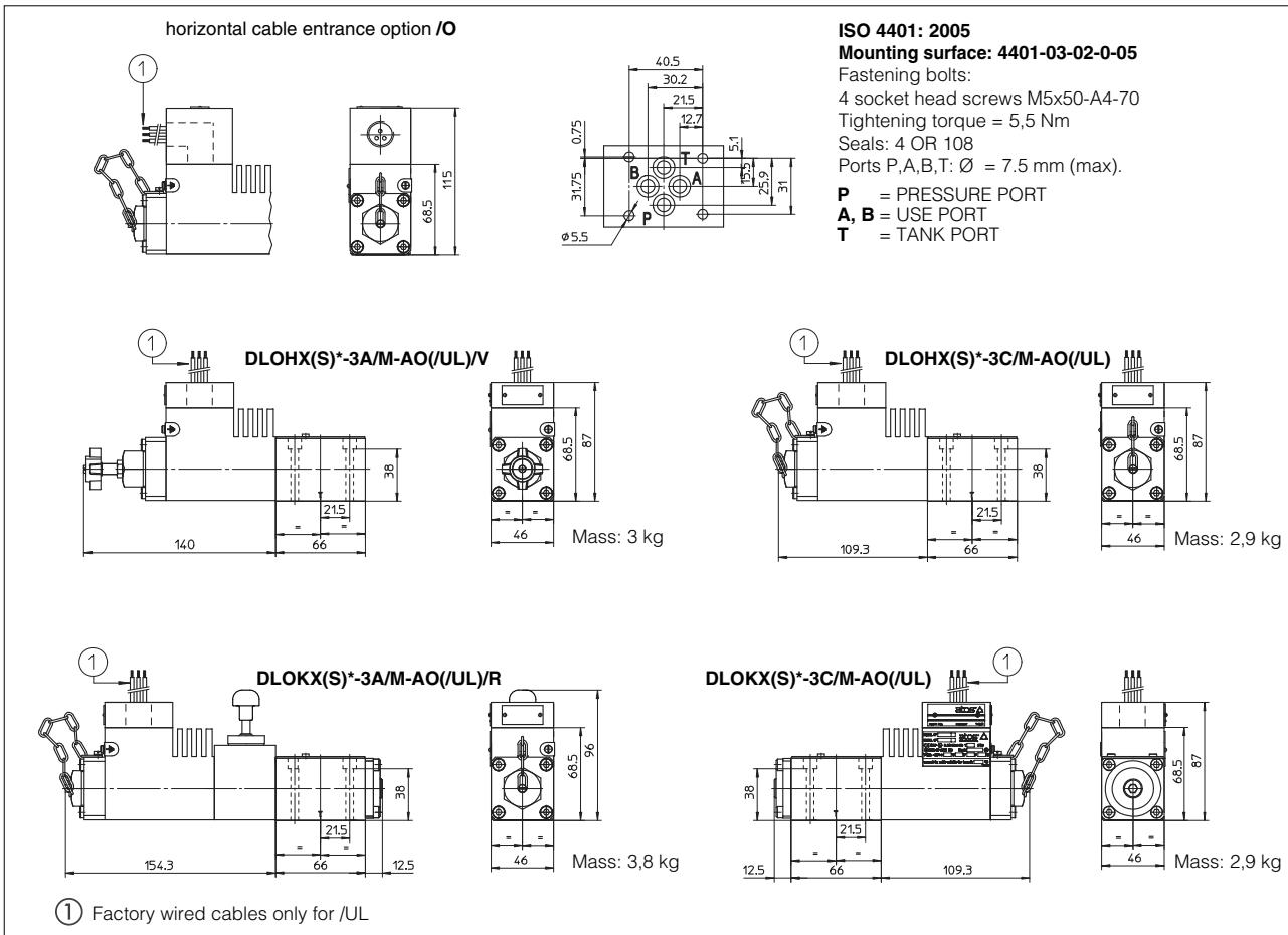
**13 INSTALLATION DIMENSIONS OF DLOPX(S) AND DLGX(S) [mm]**
