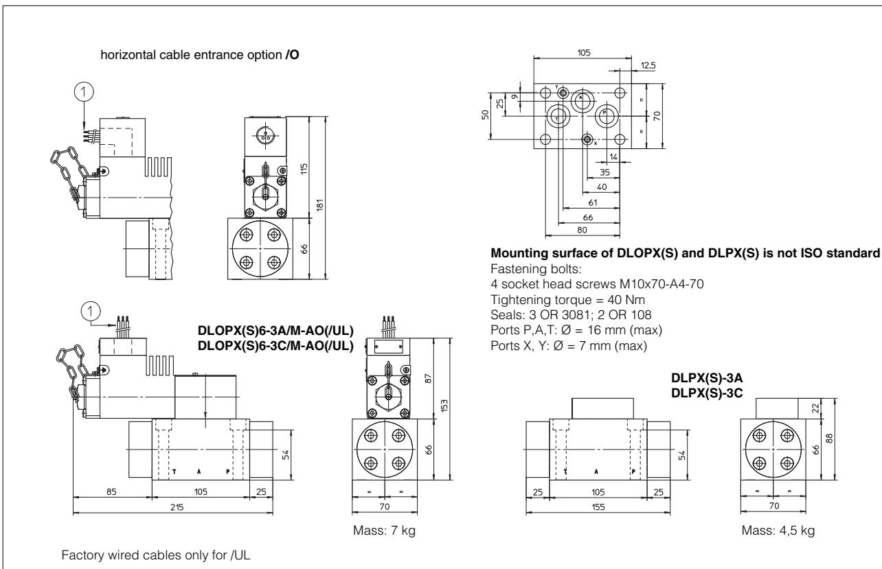
**14 INSTALLATION DIMENSIONS OF SCREW IN PRESSURE RELIEF VALVES [mm]**
