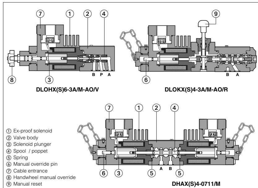
New line of directional solenoid valves and pressure relief valves in stainless steel execution for corrosive environments.
