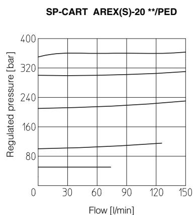
**10 PERMITTED WORKING RANGES** of screw-in cartridge valves with PED option (shared area)
