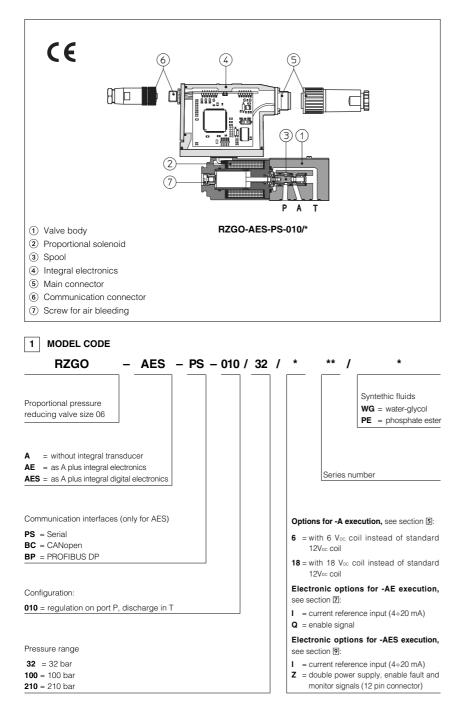
RZGO are 3-way proportional pressure reducing valves, direct operated without integral pressure transducer, which provide pressure regulation proportional to electronic reference signal.
