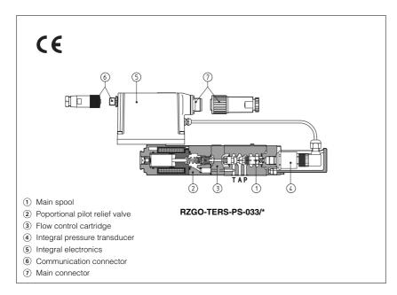
1 MODEL CODE **RZGO** - TERS - PS - 033 / 100 / reducing valve size 06 TERS = with integral digital electronics and pressure transducer AERS = as TERS but predisposed for connection of remote pressure transducer (to be ordered separately, see tab. G465) Communication interfaces
