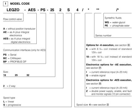
LEQZO-A\* are 2-way proportional cartridge valves, designed for mounting in manifold blocks and provide not compensated flow control according to the electronic reference signal.
