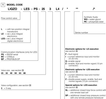
LIQZO-L\* are 3-way proportional cartridge valves, with double position transducer designed for mounting in mainfold blocks which provide both directional and non compensated flow control according to electronic reference signal.
