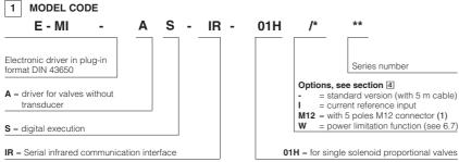
E-MI-AS digital drivers are designed for mounting on the solenoid's DIN connector of proportional valves without transducer. They supply and control the current to the solenoid according to the electronic reference input signal. The solenoid proportionally transforms the current into a force, acting on the valve spool or poppet, against a reacting spring, thus providing the valve's hydraulic regulation.
