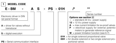
E-BM-AS digital drivers supply and control the current to the solenoid of Atos proportional valves without transducer, according to the electronic reference input signal. The solenoid proportionally transforms the current into a force, acting on the valve spool or poppet, against a reacting spring, thus providing the hydraulic regulation.
