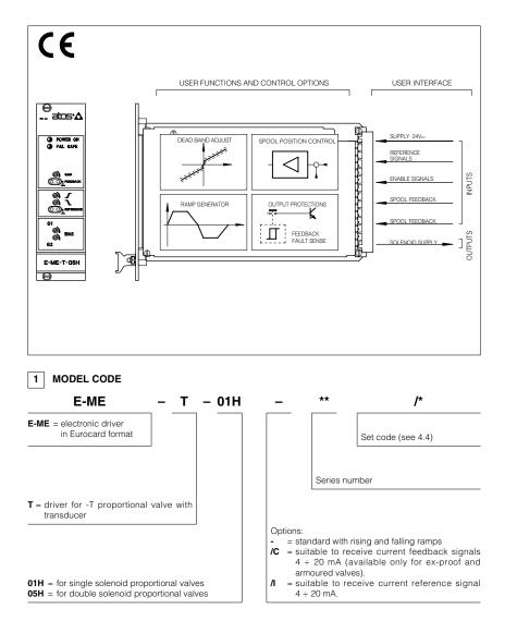
E-ME-T drivers control the current to the solenoid of Atos proportional valves with position transducer, regulating the spool position or the flow according to the electronic reference signal, adjusted by transducer's feedback.
