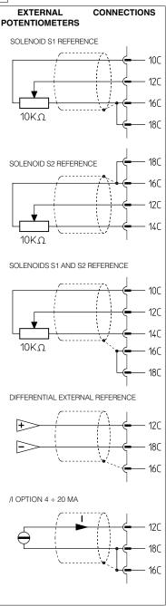
The two available regulations P3 and P4 permit to respectively regulate the ramp times for positive and negative variations of the reference signal. In case of application of the driver in closed loop systems, it is advisable to disable the ramp function: it is possible to permanently disable this function by means of a switch on the card side  $(\boxed{2})$  or temporarily, connecting the pin 6c and 6a  $(\boxed{2})$
