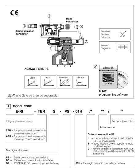
Note: the set code identifies the correspondance between the digital integral driver and the relevant valve; it is assigned by Atos when the driver is ordered as spare a part.
