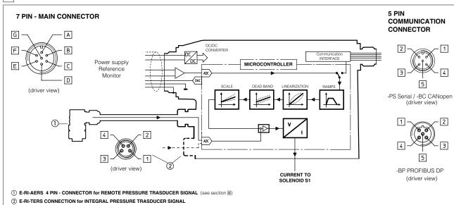
These integral digital drivers ① supply and control, in closed loop, the regulated pressure of direct and pilot operated proportional valves according to the electronic reference input signal.
