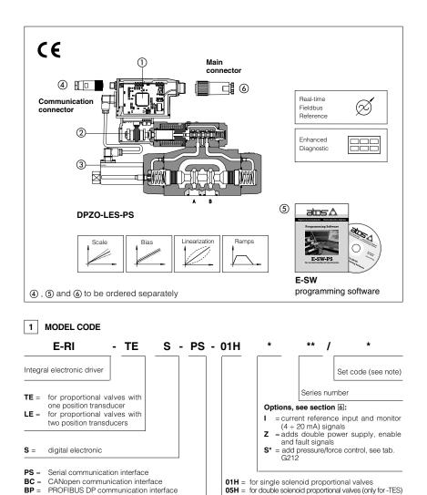
Note: the set code identifies the correspondance between the digital integral driver and the relevant valve; it is assigned by Atos when the driver is ordered as a spare part
